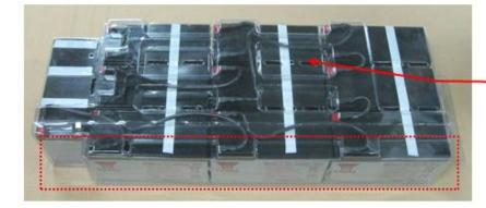
Batt. Wire should be placed in the slot of top cover.
