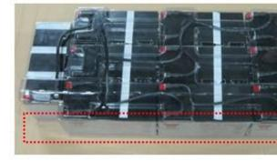
The batt. Wire should be out of the top cover through the hole.
